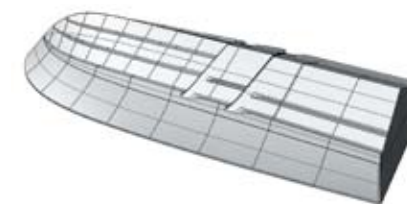
Before Peters came along with his soft-riding stepped hull, offshore boats with steps were, at best, sketchy to handle at high speeds.
